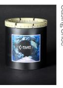
The importance of shoes is often overlooked, but as they lie at the very start of a drilling job, their reliability is of prime importance. Shoes are designed to be robust to withstand the rigours of advancing the drill string through overburden and into bedrock; as such they are reinforced with carbide and thermally stable diamonds on both the inside and outside gauges—a feature not shared by every competitor.
